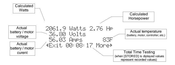
You are now able to measure Watts, amps, volts, temperature and even horsepower. Pressing the right button will allow you to toggle into the **[STORED]** mode which will display peak amps, minimum voltage, max temperature as well as the calculated watts and horsepower.
