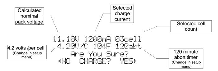
8 . The Xtrema will give you one last chance to abort before charging. It will calculate the Li voltage based on cell count and display the charge current that you have selected.
